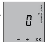
To allow the user to modify the set-point, press on the + button in Economy mode until “----” is displayed on the screen.
